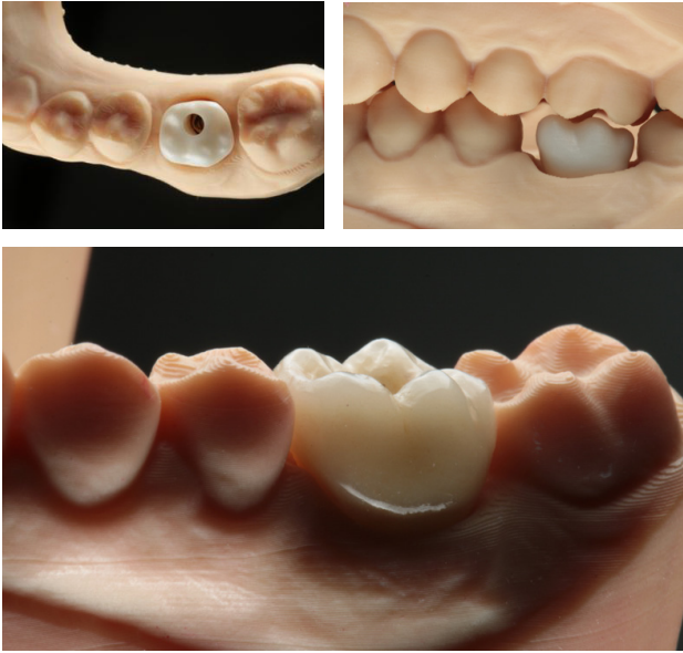
Figure 9a, b, c. 3D printed models, framework production and feldspathic veneered crown fabrication
