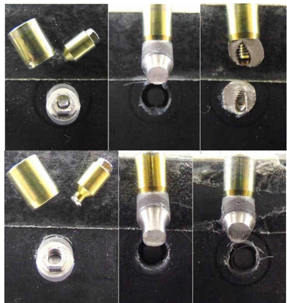
Figure 6. “Percentage of Specimens that failed under the dynamic fatigue test performed with ISO 14801 standards a) Classic-generation zygomatic implants. b) New-generation zygomatic implants
